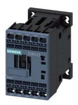
Coupling contactor relay railway 2 NO + 2 NC, 110 V DC,  $0.7 \dots 1.25^*$  US, with varistor integrated, Size S00, Spring-type terminal for upright mounting position
