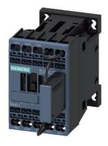
Contactor relay for railway, 2 NO + 1 NC, 110 V DC, 0.7  $\dots$  1.25\* US, with integrated varistor, 3-pole, Size S00, Spring-type terminal for upright mounting position
