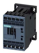
Coupling contactor relay, 2 NO + 2 NC, 24 V DC, 0.85  $\dots$  1.85\* US, with integrated suppressor diode, Size S00, Spring-type terminal
