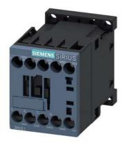
Coupling contactor relay, 3 NO + 1 NC, 24 V DC, 0.85  $\dots$  1.85\* US, with integrated diode, Size S00, screw terminal
