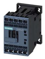
Contactor relay, 3 NO + 1 NC, 110 V AC, 50 / 60 Hz, Size S00, Spring-type terminal
