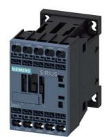
Coupling contactor relay, 3 NO + 1 NC, 24 V DC, 0.7 ... 1.25\* US, with integrated suppressor diode, Size S00, Spring-type terminal suitable for PLC outputs
