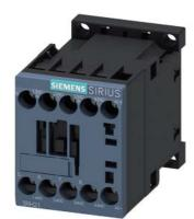
Coupling contactor relay, 4 NO, 110 V DC, 0.7 ... 1.25\* US, with integrated suppressor diode, Size S00, screw terminal suitable for PLC outputs
