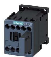
Coupling contactor relay, 4 NO, 24 V DC, 0.85  $\dots$  1.85\* US, with varistor plugged on, Size S00, screw terminal
