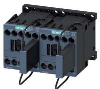
Contactor relay, latched railway, 3 NO, 32 V DC, 0.7  $\dots$  1.25\* US, with integrated varistor, and series resistor, Size S00, screw terminal
