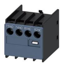
Auxiliary switch on the front, 1 NO + 1 NC Current path 1 NO, 1 NC Connection from top for 3RH and 3RT screw terminal 73/74, 81/82
