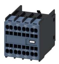
Auxiliary switch on the front, 1 NO + 3 NC Current path 1 NO, 1 NC, 1 NC, 1 NC for contactor relays Size S00 spring-type terminal 51/52, 61/62, 71/72, 81/82 Physically coded; only with contactor relays 3RH2140\* and 3RH2440\* can be combined (according to EN 50011)
