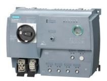
SIRIUS motor starter M200D AS-i Communication: AS-Interface DOL starter Basic Mechanical switching AC-3, 0.75KW / 400 V 0.15 A...2.00 A Electronic overload protection Thermistor: THERMOCLICK / PTC without brake contact 2DI AS-i + 2DI / 1DO on device Han Q4/2 - Han Q8/0
