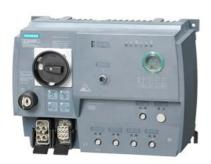
SIRIUS motor starter M200D AS-i Communication: AS-Interface DOL starter Basic Mechanical switching AC-3, 5.5 kW / 400 V 1.5 A...12.00 A Electronic overload protection Thermistor: THERMOCLICK / PTC without brake contact 2DI AS-i + 2DI / 1DO on device Han Q4/2 - Han Q8/0 with manual on-site operation and key-operated switch
