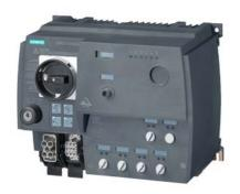
SIRIUS motor starter M200D AS-i Communication: AS-Interface Reversing starter standard Mechanical switching AC-3, 0.75KW / 400 V 0.15 A...2.00 A Electronic overload protection Thermistor: THERMOCLICK / PTC without brake contact 4 DI / 1 DO AS-i Han Q4/2 - Han Q8/0 with manual on-site operation and key-operated switch
