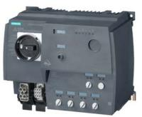
SIRIUS motor starter M200D AS-i Communication: AS-Interface DOL starter Standard Electronic switching AC-3, 0.75KW / 400 V 0.15 A...2.00 A Electronic overload protection Thermistor: THERMOCLICK / PTC without brake contact 4 DI / 1 DO AS-i Han Q4/2 - Han Q8/0
