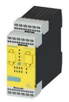
SIRIUS, Central unit 3RK3 ASIsafe Extended for modular Safety system 3RK3 2/4 F-DI, 4 DI, 1 F-RO, 1 F-DO,24 V DC Monitoring of ASI slaves Control of 10 safe outputs on AS-Interface bus parameterizable using software Safety ES 45 mm overall width Spring-type terminal Up to SIL3 (IEC 61508) Up to Performance Level E (ISO 13849-1) 2 extension modules connectable
