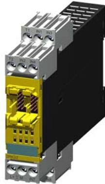
SIRIUS, Extension module 3RK32 for modular Safety system 3RK3 2/4 F-DI, 2 F-DO, 24 V DC/1.2 A Can be parameterized via MSS ES 22.5 mm overall width screw terminal Up to SIL3 (IEC 61508) Up to Performance Level E (ISO 13849-1) without connection cable
