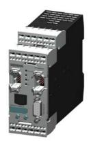
SIRIUS, interface module DP interface, for modular safety system 3RK3 PROFIBUS DP interface 12 Mbps, RS 485 45 mm overall width spring-type terminal can be parameterized via Safety ES without connection cable
