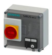
SIRIUS MCU motor starter Enclosure degree of protection IP55 plastic Communication without electromechanically switching Short-circuit protection with circuit breaker DOL starter Brake without Performance class 12 A Motor circuit breaker with bi-metal thermal Manual operation latching Connection power M screw connection Electrical wholesale version
