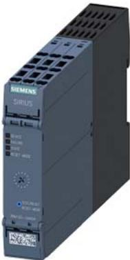
Reversing starter, 3RM1, 500 V, 0.09 - 0.75 kW, 0.4 - 2 A, 24 V DC, spring-type terminals
