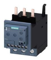
Monitoring relay, can be mounted to Contactor 3RT2, Size S2 basic, analog adjustment Apparent current monitoring 8...80 A, 50...60 Hz, 2-phase Supply 24 V AC/DC 1 change-over contact Monitoring for Current overshoot and undershoot Phase failure, Cable break with or without fault buffer ON delay 0-60 s Noise pulse suppression 0-30 s Switching hysteresis 6% Screw connection system
