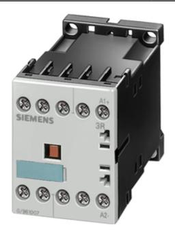
COUPLING RELAY, AC-3 4 KW/400 V, 1 NC, DC 24 V, 0.7...1.25\*US, 3-POLE, SIZE S00, SCREW CONNECTION
