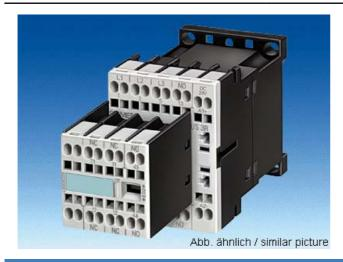
COUPLING RELAY, AC-3 4 KW/400 V, 1 NC, DC 24 V, 0.7...1.25\*US, 3-POLE, SIZE S00, CAGE CLAMP CONNECTION
