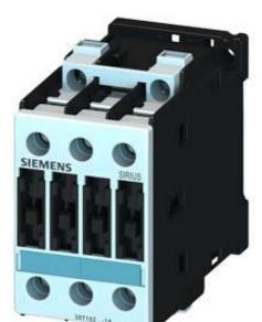
Power contactor, AC-3 17 A, 7.5 kW / 400 V 110 V AC, 50 Hz / 120 V, 60 Hz 3-pole, Size S0 Screw terminal !!! Phased-out product !!! Successor is SIRIUS 3RT2 Preferred successor type is >>3RT2025-1AK60<<
