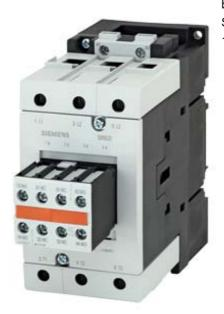
Power contactor, AC-3 80 A, 37 kW / 400 V 230 V AC, 50 Hz 2 NO + 2 NC, 3-pole, Size S3, Screw terminal Front-side auxiliary switch block captive for SUVA applications !!! Phased-out product !!! Successor is SIRIUS 3RT2 Preferred successor type is >>3RT2038-1CL24-3MA0<<
