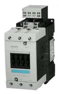
Power contactor, AC-3 95 A, 45 kW / 400 V 24 V DC, 0.7-1.25\* Us 3-pole, Size S3 Spring-type terminal With electronic control unit Integrated varistor !!! Phased-out product !!! Successor is SIRIUS 3RT2 Preferred successor type is >>3RT2046-3XB40-0LA2<<
