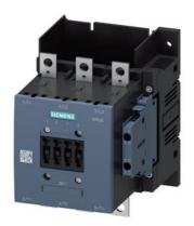
power contactor, AC-3e/AC-3 115 A, 55 kW / 400 V, without operating mechanism 3-pole, auxiliary contacts 2 NO + 2 NC drive: conventional main circuit: busbar control and auxiliary circuit: screw terminal
