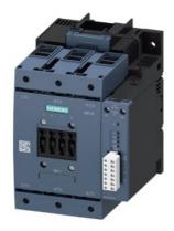
power contactor, AC-3e/AC-3 115 A, 55 kW / 400 V, AC (50-60 Hz) / DC Uc: 96-127 V PLC input 24 V DC 3-pole, auxiliary contacts 1 NO + 1 NC drive: electronic main circuit: box terminal control and auxiliary circuit: screw terminal , remaining lifetime signal
