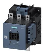
power contactor, AC-3e/AC-3 115 A, 55 kW / 400 V, AC (50-60 Hz) / DC Uc: 110-127 V 3-pole, auxiliary contacts 2 NO + 2 NC drive: conventional main circuit: busbar control and auxiliary circuit: spring-loaded terminal
