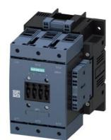
power contactor, AC-3e/AC-3 115 A, 55 kW / 400 V, AC (50-60 Hz) / DC Uc: 440-480 V 3-pole, auxiliary switch right 3RH1921-2DE11 drive: conventional main circuit: box terminal control and auxiliary circuit: spring-loaded terminal
