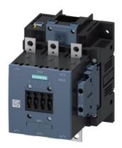
power contactor, AC-3e/AC-3 115 A, 55 kW / 400 V, AC (50-60 Hz) / DC Uc: 96-127 V PLC input 24 V DC 3-pole, auxiliary contacts 2 NO + 2 NC drive: electronic main circuit: busbar control and auxiliary circuit: screw terminal
