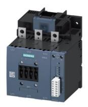
power contactor, AC-3e/AC-3 115 A, 55 kW / 400 V, AC (50-60 Hz) / DC Uc: 96-127 V PLC input 24 V DC 3-pole, auxiliary contacts 1 NO + 1 NC drive: electronic main circuit: busbar control and auxiliary circuit: screw terminal , remaining lifetime signal
