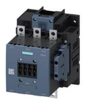
power contactor, AC-3e/AC-3 150 A, 75 kW / 400 V AC (50-60 Hz) / DC Uc: 23-26 V 3-pole, auxiliary contacts 2 NO + 2 NC drive: conventional main circuit: busbar control and auxiliary circuit: screw terminal
