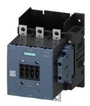
power contactor, AC-3e/AC-3 150 A, 75 kW / 400 V without operating mechanism 3-pole, auxiliary contacts 2 NO + 2 NC without operating mechanism main circuit: busbar control and auxiliary circuit: screw terminal
