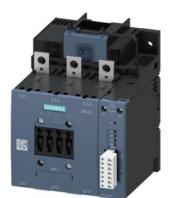
power contactor, AC-3e/AC-3 150 A, 75 kW / 400 V AC (50-60 Hz) / DC Uc: 96-127 V PLC input 24 V DC 3-pole, auxiliary contacts 1 NO + 1 NC drive: electronic main circuit: busbar control and auxiliary circuit: screw terminal with remaining lifetime indicator
