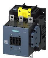
power contactor, AC-3e/AC-3 150 A, 75 kW / 400 V AC (50-60 Hz) / DC Uc: 96-127 V x (0.8-1.1) F-PLC input 24 V DC 3-pole, auxiliary contacts 2 NO + 2 NC drive: electronic main circuit: busbar control and auxiliary circuit: screw terminal
