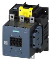
power contactor, AC-3e/AC-3 150 A, 75 kW / 400 V AC (50-60 Hz) / DC Uc: 200-277 V x (0.8-1.1) F-PLC input 24 V DC 3-pole, auxiliary contacts 2 NO + 2 NC drive: electronic main circuit: busbar control and auxiliary circuit: screw terminal
