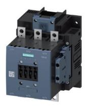
power contactor, AC-3e/AC-3 185 A, 90 kW / 400 V AC (50-60 Hz) / DC Uc: 23-26 V 3-pole, auxiliary contacts 2 NO + 2 NC drive: conventional main circuit: busbar control and auxiliary circuit: screw terminal
