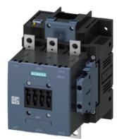
power contactor, AC-3e/AC-3 185 A, 90 kW / 400 V AC (50-60 Hz) / DC Uc: 200-277 V PLC input 24 V DC 3-pole, auxiliary contacts 2 NO + 2 NC drive: electronic main circuit: busbar control and auxiliary circuit: screw terminal
