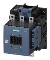
power contactor, AC-3e/AC-3 185 A, 90 kW / 400 V Uc: 72 V DC x (0.7-1.25) PLC input 24-110 V DC 3-pole, auxiliary contacts 2 NO + 2 NC drive: electronic main circuit: busbar control and auxiliary circuit: spring-loaded terminal extended rated condition railroad IEC 60077
