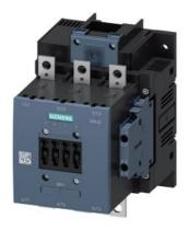
power contactor, AC-3e/AC-3 185 A, 90 kW / 400 V AC (50-60 Hz) / DC Uc: 500-550 V 3-pole, auxiliary contacts 2 NO + 2 NC drive: conventional main circuit: busbar control and auxiliary circuit: screw terminal
