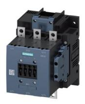
contactor, 100HP, 460 / 575 V AC (50...60 Hz) / DC operation 575 ... 600 V AC/DC auxiliary contacts 2 NO + 2 NC 3-pole, frame size S6 busbar connections drive: conventional NEMA size 4
