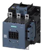
power contactor, AC-3e/AC-3 185 A, 90 kW / 400 V AC (50-60 Hz) / DC Uc: 21-27, 3 V PLC input 24 V DC 3-pole, auxiliary contacts 2 NO + 2 NC drive: electronic main circuit: busbar control and auxiliary circuit: screw terminal
