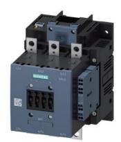
power contactor, AC-3e/AC-3 185 A, 90 kW / 400 V AC (50-60 Hz) / DC Uc: 200-277 V PLC input 24 V DC 3-pole, auxiliary contacts 2 NO + 2 NC solid-state compatible drive: electronic main circuit: busbar control and auxiliary circuit: screw terminal
