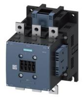
power contactor, AC-3e/AC-3 225 A, 110 kW / 400 V AC (50-60 Hz) / DC Uc: 110-127 V 3-pole, auxiliary contacts 2 NO + 2 NC drive: conventional main circuit: busbar control and auxiliary circuit: spring-loaded terminal
