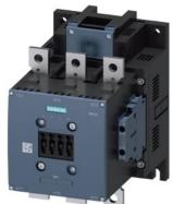
power contactor, AC-3e/AC-3 225 A, 110 kW / 400 V AC (50-60 Hz) / DC Uc: 110-127 V 3-pole, auxiliary contacts 2 NO + 2 NC drive: conventional main circuit: busbar control and auxiliary circuit: screw terminal
