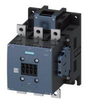
power contactor, AC-3e/AC-3 225 A, 110 kW / 400 V AC (50-60 Hz) / DC Uc: 200-220 V 3-pole, auxiliary contacts 2 NO + 2 NC drive: conventional main circuit: busbar control and auxiliary circuit: screw terminal
