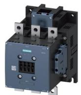
power contactor, AC-3e/AC-3 225 A, 110 kW / 400 V AC (50-60 Hz) / DC Uc: 96-127 V PLC input 24 V DC 3-pole, auxiliary contacts 2 NO + 2 NC drive: electronic main circuit: busbar control and auxiliary circuit: screw terminal
