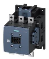
power contactor, AC-3e/AC-3 225 A, 110 kW / 400 V AC (50-60 Hz) / DC Uc: 200-277 V PLC input 24 V DC 3-pole, auxiliary contacts 2 NO + 2 NC drive: electronic main circuit: busbar control and auxiliary circuit: screw terminal
