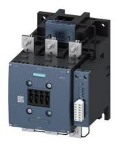
power contactor, AC-3e/AC-3 225 A, 110 kW / 400 V AC (50-60 Hz) / DC Uc: 96-127 V PLC input 24 V DC 3-pole, auxiliary contacts 1 NO + 1 NC drive: electronic main circuit: busbar control and auxiliary circuit: screw terminal with remaining lifetime indicator
